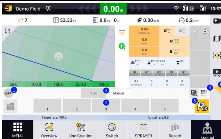
Figure 38 Spray system status window-TC
